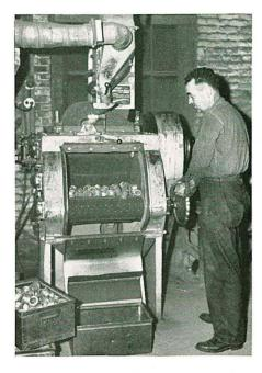
15" x 20" Wheelabrator Tumblast cleaning parts for WaterFOG nozzles.
